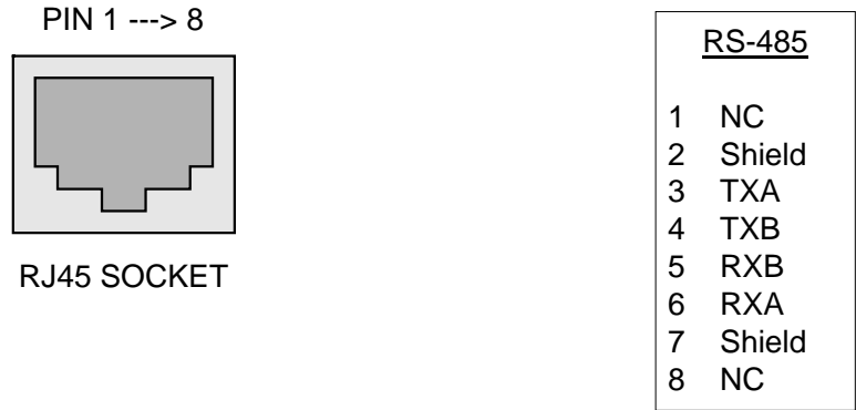
Figure 3: Pin Definition of RJ45
